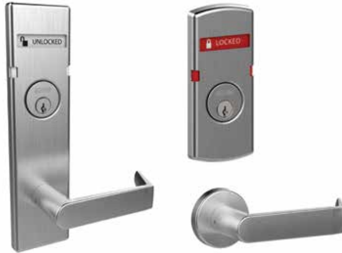
With a classroom security lockset, a staff member with a key can lock the outside lever without opening the classroom door. The inside lever always allows free egress. An indicator on the lock gives a visual indication of the door status.
